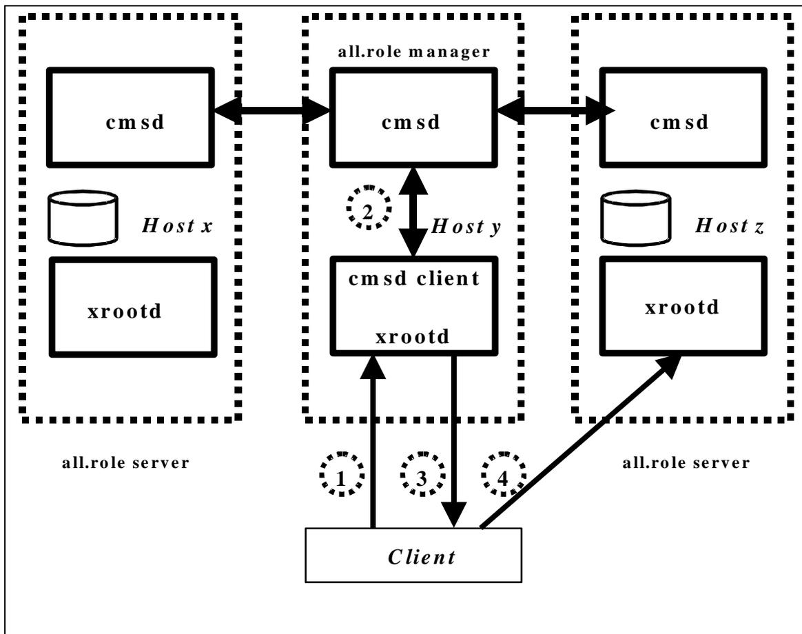
In the diagram, there are three hosts: *x*, *y*, and *z*. Host *y* serves as the load balancer. Hosts *x* and *z* are the hosts that can be used to serve data to clients and load is to be distributed between the two. Consequently, host *y* runs a manager **cmsd** while hosts *x* and *z* run server **cmsd**'s.
