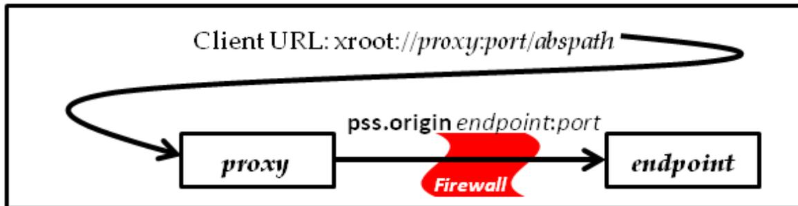
In the diagram the client present a URL that identifies the proxy server or proxy cluster. The proxy then contacts the data origin, a particular endpoint, on behalf of the client and performs the requested operation. The endpoint can be an actual server or a cluster redirector. This mode is suitable for incoming connections to a fire walled cluster or outgoing connections to a particular data source.
